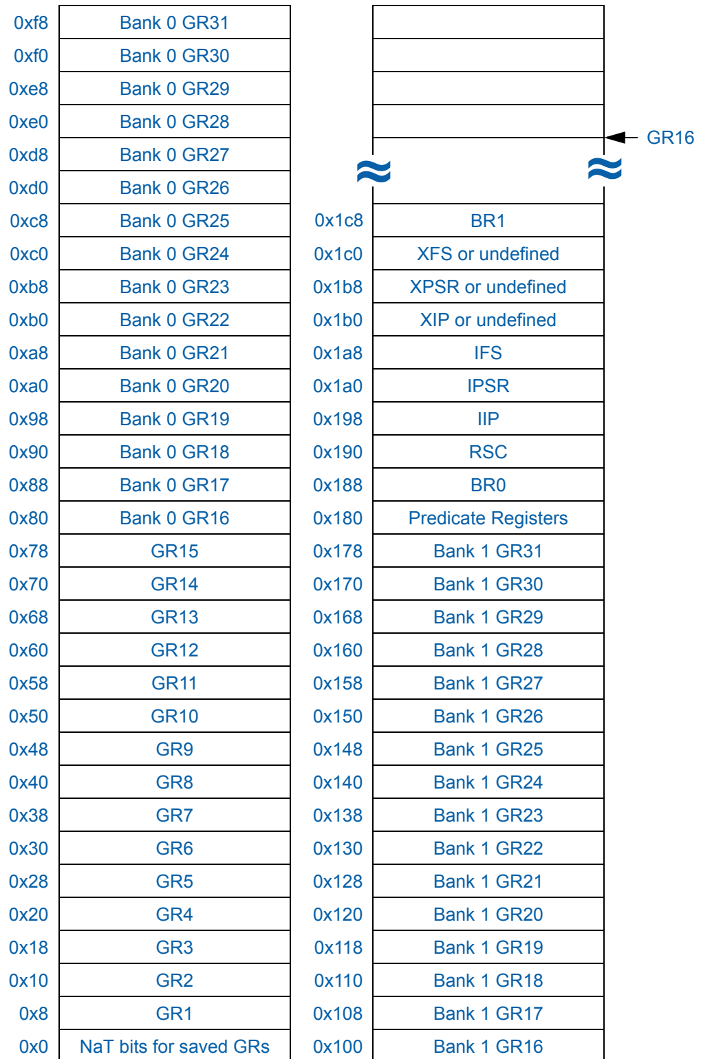
Figure 11-2. Processor State Saved in Min-state Save Area
